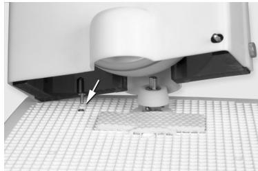
6) Swivel the band saw attachment so that the drive roller touches the drive cone. Fasten the elastic band so that it stretches from the lateral pin to the grid plate. This will create a constant pressure onto the drive cone.
