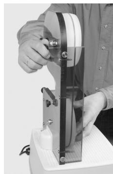
10) Without pressure, tighten the eccentric below the rocker bar. Finally, put the hood and the worktable back in place and tighten the fastening screws.
