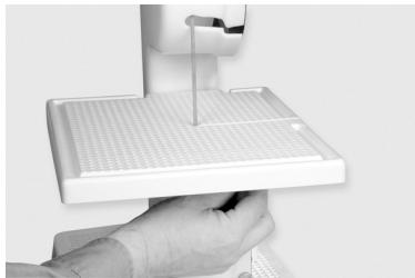
5) On the underside of the saw attachment is a pin, 10 mm long. When mounting the band saw onto the grinder, make sure that the pin is inserted into the sleeve.
