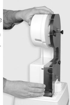
8) Place the new saw blade onto the middle of the lower band roller. Push down the upper band roller and put the saw blade onto it as well.
